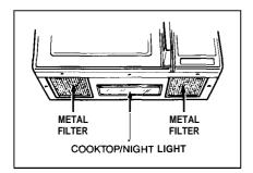
The exhaust hood feature on your microwave oven is equipped with two metal filters which collect grease. When the fan is operated, air is drawn up through the filters and is then discharged through the provided venting to the outside. The hood also has a light for illuminating the counter space.
